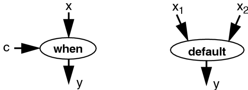
Figure 7. SIGNAL kernel constructs influencing the control execution flow
